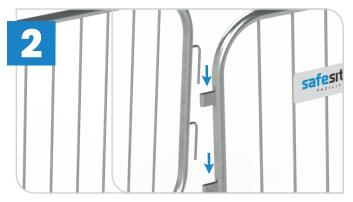
To connect the next barrier, place the hooks from one panel, into the loops of the barrier already positioned in place. Make sure that each panel faces the same direction.
